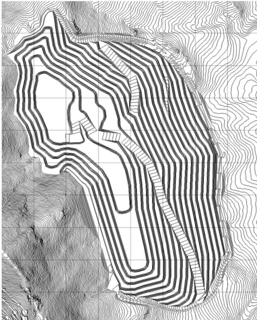
Figure 16-17: ROM Final Stacking Design
